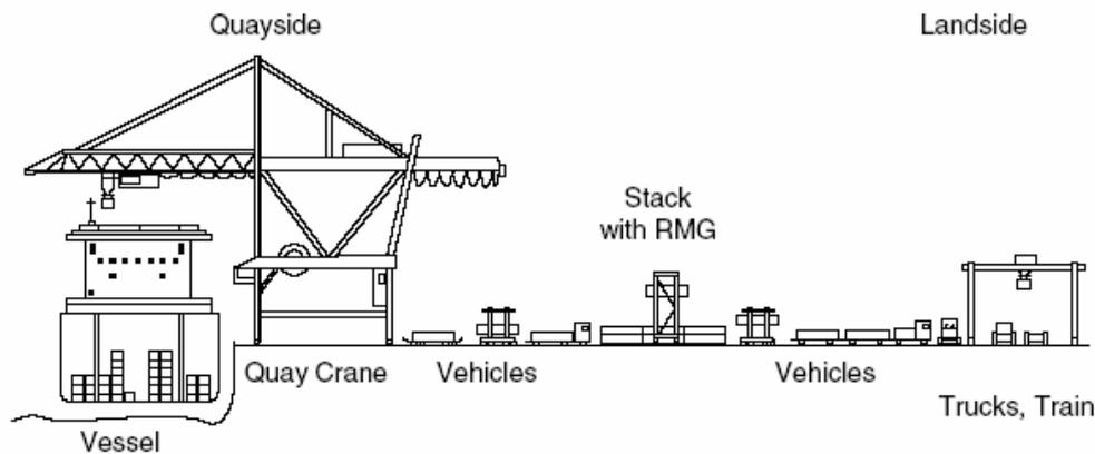
**Figure 1.** Transportation and handling chain of a container [1]
